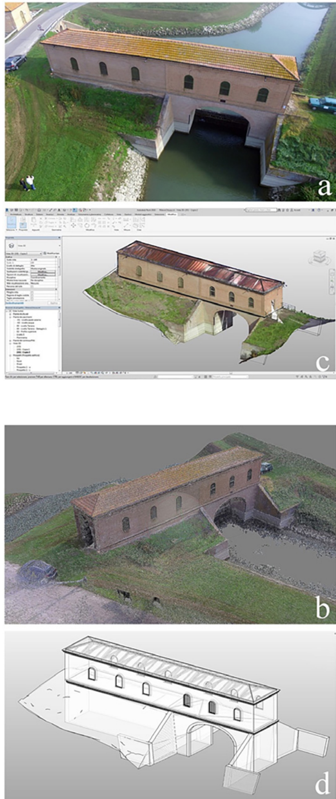
Figure 2: The most common authoring workflow to get digital BIM models from UAV digital photogrammetry. The real building (a), the registered point cloud processed from aerial pictures (b), the BIM abstraction authored translating the point cloud into a semantic object taking advantage of a BIM software environment (c), the final digital model meant to index embedded data about preservation of materials, as-built documents, structural simulation results and so forth (d) (Survey campaign, data processing and BIM model of a built sluice close to the Po river by S. Garagnani, 2016).
