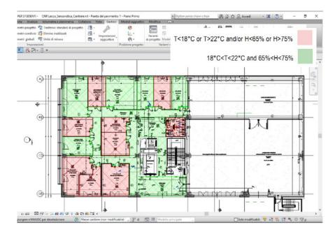
Table 1: Example of data of air temperature and relative humidity collected by field sensors in the construction site. Figure 2: Colour code to underline the levels of temperature and relative humidity.
