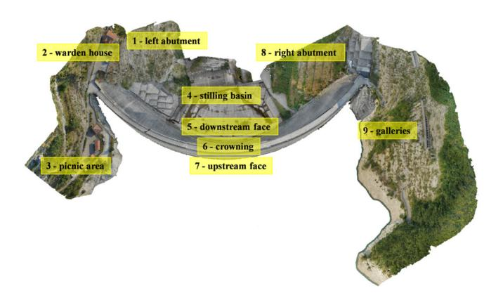
is governed by their geometry, with a maximum capacity of 600m³/s. During overflow, the flowing water dissipates its energy in the stilling basin constructed at the foot of the downstream face of the dam. Moreover, the dam has a middle height sluice gate, a bottom sluice gate and a depletion sluice gate.
