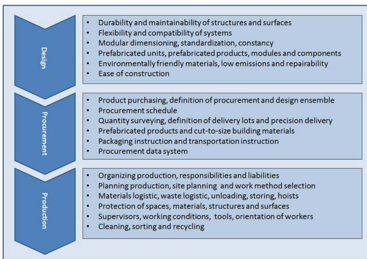
Figure 1. Focal points of improving material efficiency in three categories. Design, procurement and production. The common factor for each category is proper materials handling. (Mäkelä 2013).
