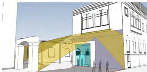
The main entry was the first real building experiment for the co-lab. The built outcome was a result of available materials and manpower. A few ladies who know how to knit shared their skills with others to create the lacy canopy; instead of typical yarn, they knit with the salvaged miles of epper wire. While connecting with the old Stoveco Arch and the new main entry, the canopy is also a community landmark, a unique example of co-labs essential and blocks of an alley was torn.
